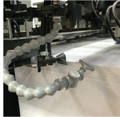
PRINTING PRESS AIR FLOW CONTROL
